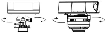
2) Release the tilt screw on both side of the device and then rotate the lens to up or down. After completion, tighten the tilt screw.
