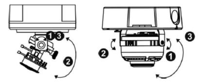
3) Release the video adjustment screw and then adjust the lens direction. After completion, tighten the video adjustment screw.
