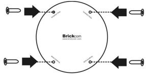
4) Mount the camera on the wall and position to four screw slots over the plastic anchors. Insert the screws into the holes and use the screwdriver to tighten the screws clockwise until they are secure.
